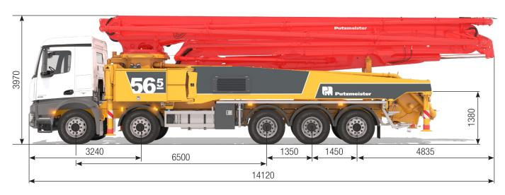
Note: Standard version. Dimensions and weights depend on truck, pump model and equipment. Dimensions in mm, MB-Actros 4640 B, Euro 2. For illustration only.
