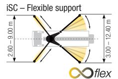
Dimensions can differ depending on configuration. Support width based on center of support leg.
